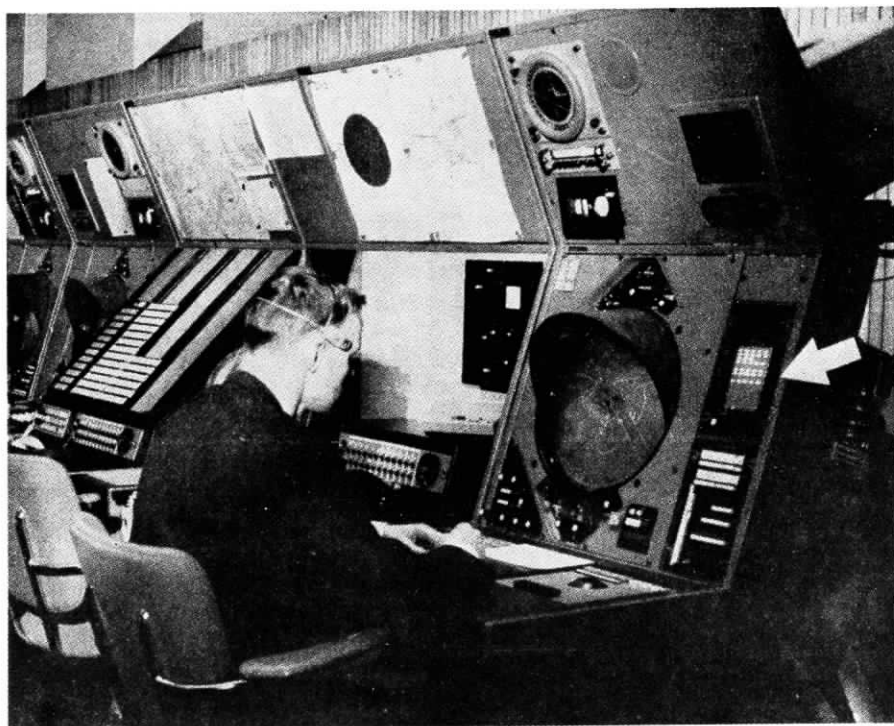
CLOSE-UP of controller position shows 16-in. cathode ray tube with area map superimposed electronically, as well as tabular display (arrow, right) which can show important flight data concerning six aircraft of interest to the controller.
